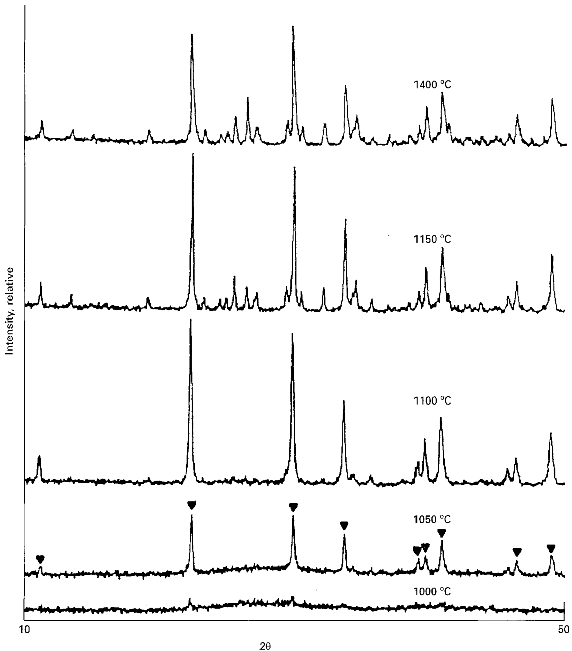
Figure 7 Powder XRD patterns of BAS bulk glass heat treated at various temperatures for 1 h. ▼ BAS hexagonal.
